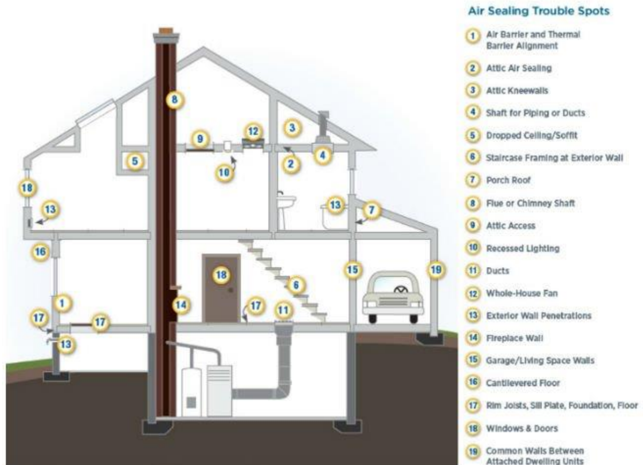
Figure 19. Example of Air sealing common trouble Spots. Source: https://www.energy.gov/energysaver/air-sealing-your-home
